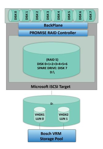
The configuration below shows an example of the centralized "all-in-one" recording, viewing and management solution for a network surveillance system of up to 128 video streams using the Promise Vess A3340 appliance.
